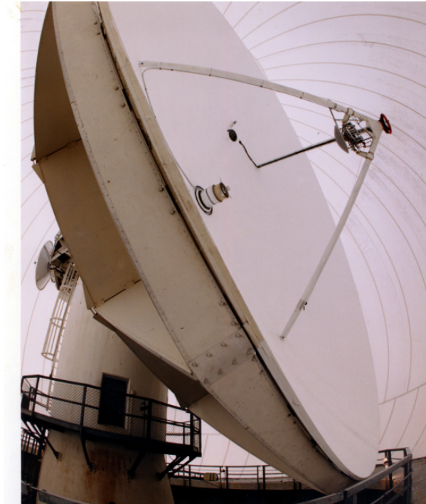
Figure 2. Wide-angle view of Westford antenna inside the radome. The VLBI S/X receiver is located at the prime focus. The subreflector in front of the receiver is installed when observing with the TAL receiver (see Section 4), which is located at the Cassegrain focus.
