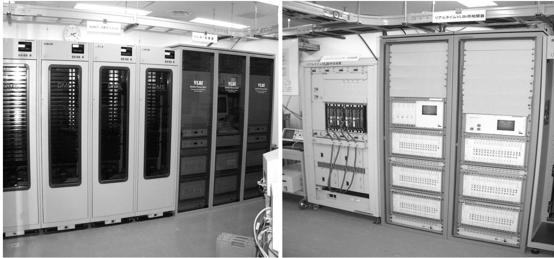
Figure 1. The KSP tape-based VLBI correlation system (left) and the KSP real-time VLBI correlation system (right) at Koganei. In the left figure, four racks at the left are automatic tape changer (DMS-24). The right three racks contain correlators, output interfaces, and correlation controller. All of these tape-based equipment will be transported to Kashima Space Research Center in near future.
