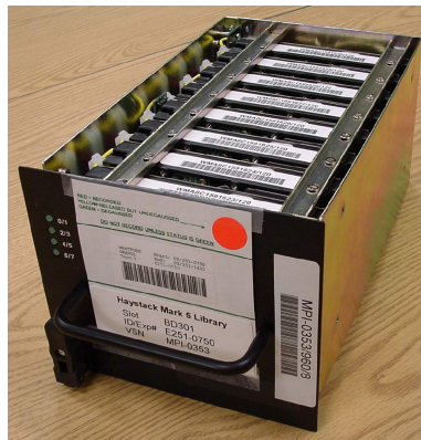
Figure 1. Mark 5A '8-pack' disk module with typical labeling
