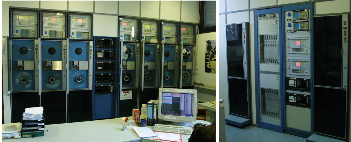
Figure 1. Tape drives with stations units on top, Mark 5 units in a rack, and the correlator surrounded by two more tape drives, Mark 5 units, and station units. The correlator control console is visible on the desk in the center.
