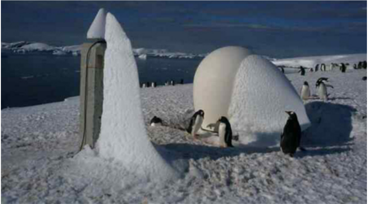
Figure 2. View from the telescope to the Ashtech GPS antenna and to the radome for the Turbo Rogue antenna.
