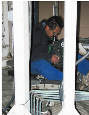
Figure 3. Jaques Grobler operating the theodolite located in the "elephant base" during the night alignment.
