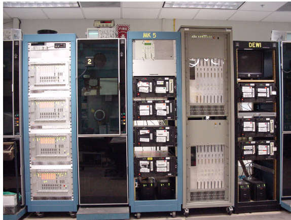
Figure 1. Partial view of the Haystack Mark IV correlator, showing 2 racks containing 7 Mark 5A units and a decoder, correlator rack, 1 tape unit, and 1 rack containing 4 Station Units.
