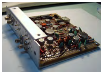
Figure 2. Prototype of the Cable Length Calibration System Ground Unit (without phase comparator)
