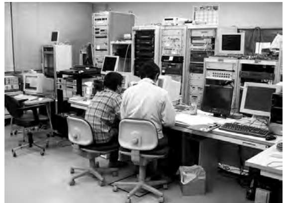
Figure 1. A view of the observation room of Kashima 34m antenna. K5 system located in this room is used for observation and also for correlation processing.
