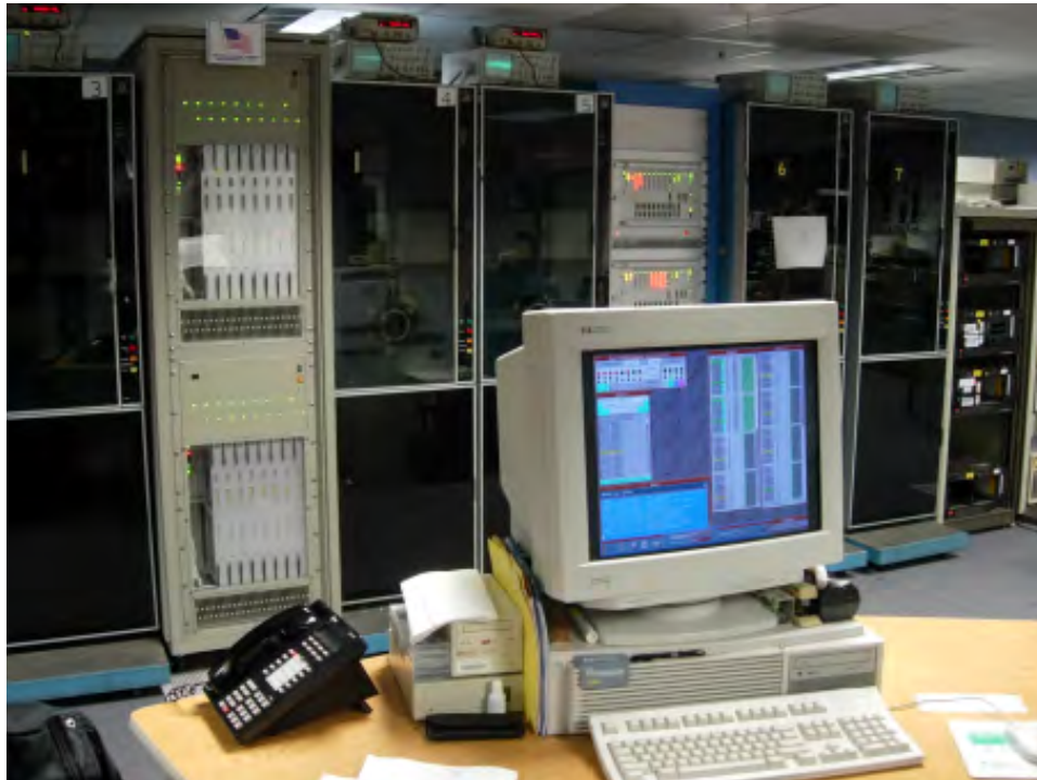
Figure 1. The right half of WACO showing 4 Mark 5A units (far right), legacy tape drives, the operator's console, and the central processor (left).
