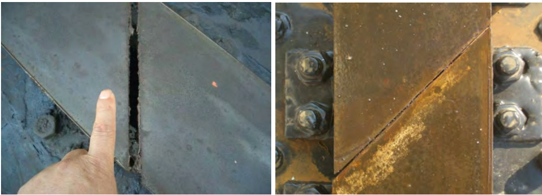
Figure 1. Left: deformation in the rail of the Sheshan 25m telescope (photo taken on 8 August 2006). Right: reconstructed tracks (photo taken on 25 December 2006).
