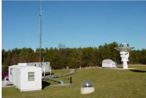
Figure 2. New permanent MV3 antenna.
