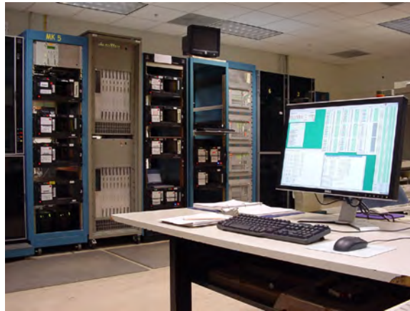
Figure 1. Partial view of the Haystack Mark IV correlator, showing 3 racks containing 7 Mark 5A correlator playback units, 2 Mark 5B DOM correlator playback units with associated correlator interface board units, 1 Mark 5A e-VLBI transfer unit, decoder, the correlator rack, 3 tape drives, and 1 rack containing 4 Station Units. In the foreground is the new linux-based correlator control computer display.
