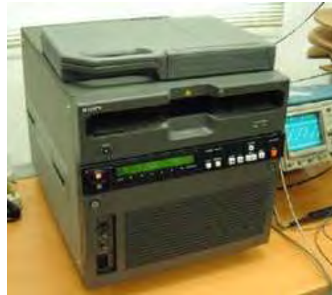
Figure 3. DIR2000: 1 Gbps recorder used in VERA operations.
