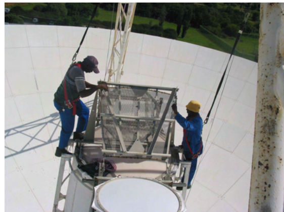
Figure 2. Andrew Masiteng and Richard Moralo install the dichroic reflector, which permits simultaneous observing at 3.5 and 13 cm. The dichroic has to be installed before and removed after every geodetic VLBI experiment.
