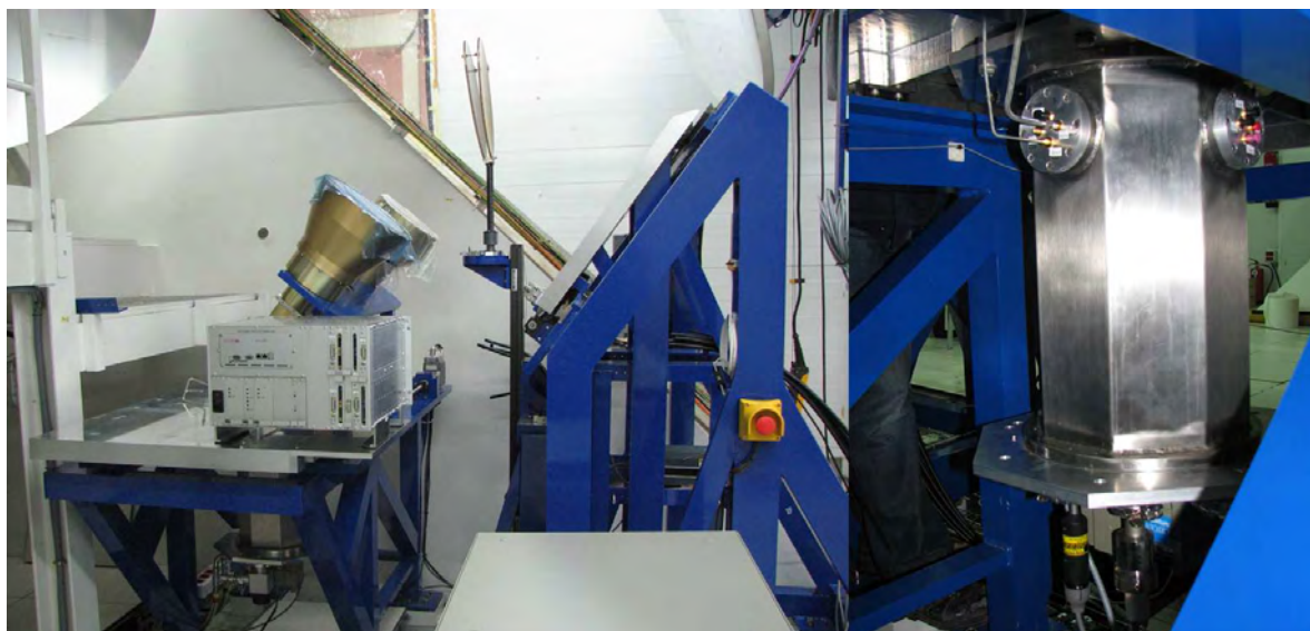
Figure 2. Photograph of the new S/C/CH-bands receiver, installed at the new 40-m radiotelescope cabin.
