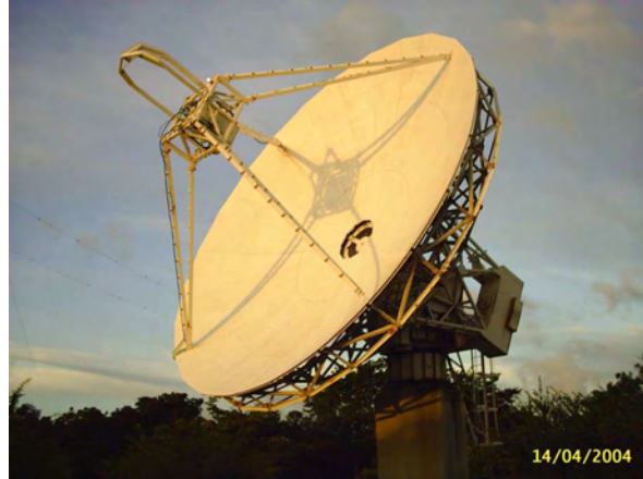
Figure 1. Fortaleza's 14.2 m antenna.
