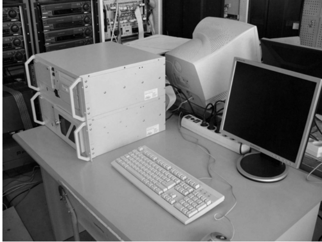
Figure 1. 12-board MicroPARSEc correlator.
