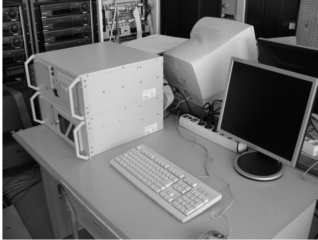
Figure 1. 12-board MicroPARSEc correlator.
