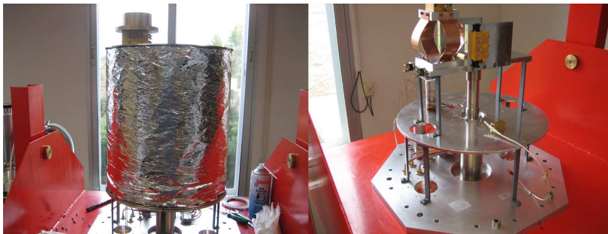
Figure 1. Photograph of the new X-band receiver, to be installed at the new 40-m radiotelescope.
