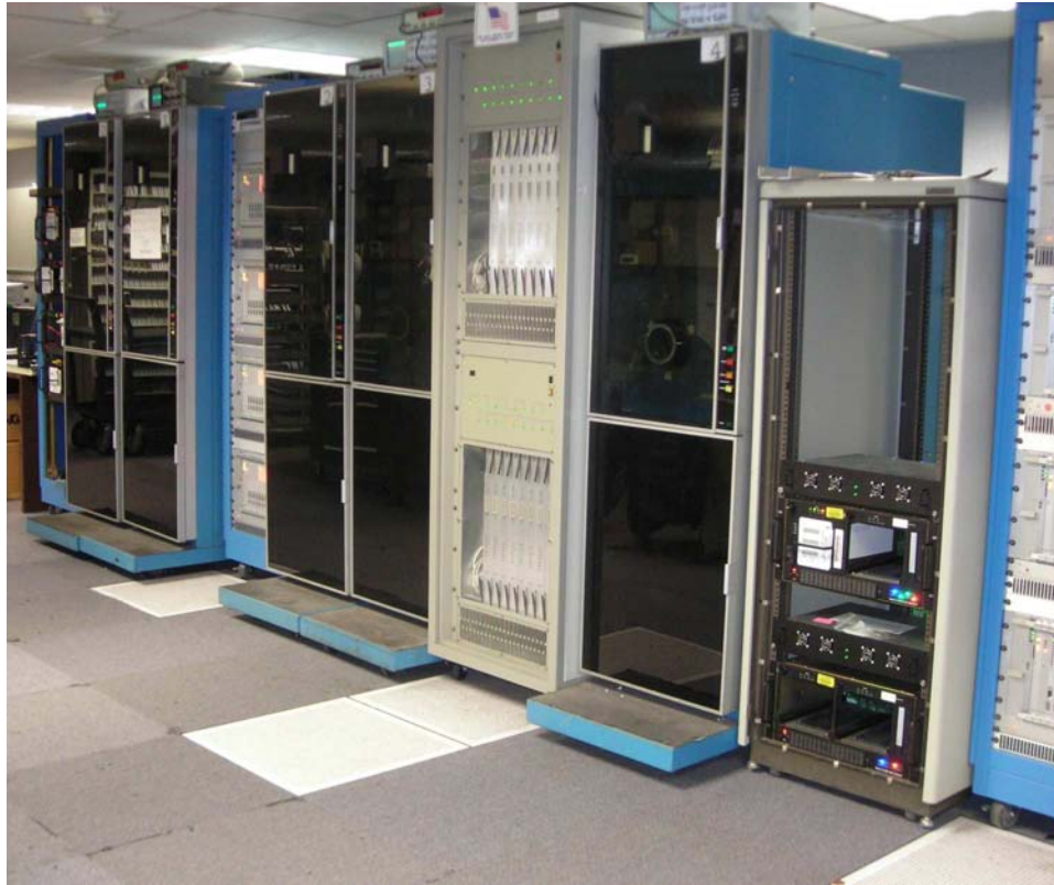
Figure 1. The WACO Mark IV Correlator, showing the Mark 5B units (right), legacy tape drives (no longer used), the central processing rack and beyond it one of two station unit racks. The far left rack contains four Mark 5A units and the broadband Internet terminal.
