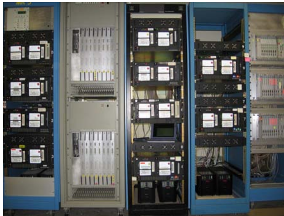
Figure 1. Partial view of the Haystack Mark IV correlator, showing five racks containing (left to right) four Mark 5A correlator playback units, the Mark IV correlator, three Mark 5A correlator playback units, and one Mark 5B correlator playback unit (bottom) with the associated correlator interface board unit, two Mark 5B correlator playback units with associated correlator interface board units, and three station units.
