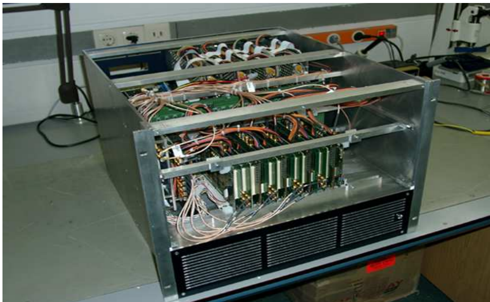
Figure 1. DBBC internal view
