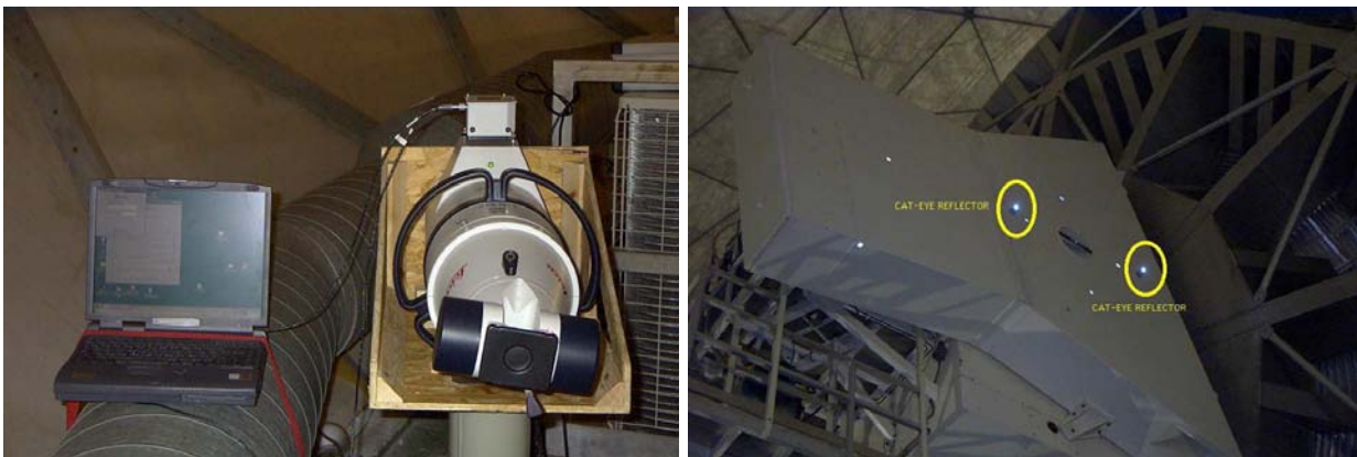
Figure 2. Left: the laser tracker mounted on a survey pillar inside the radome building of the 20 m telescope. Right: cat-eye reflectors mounted on the telescope cabin.
