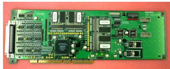
Figure 2. VSI-card can record high-bandwidth data to commodity PC.
