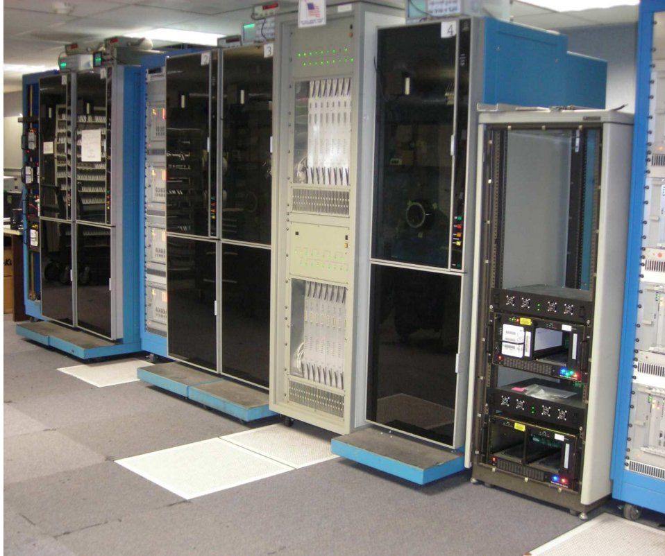
Figure 1. The WACO Mark IV Correlator, showing the Mark 5B units (right), legacy tape drives (no longer used), the central processing rack and beyond it one of two station unit racks. The far left rack contains four Mark 5A units and the broadband Internet terminal.
