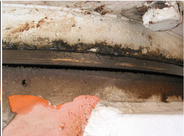
Figure 2. The 26-m telescope breaks down. The gap between the bearing housing and static ring confirms suspicion of a south polar bearing collapse.
