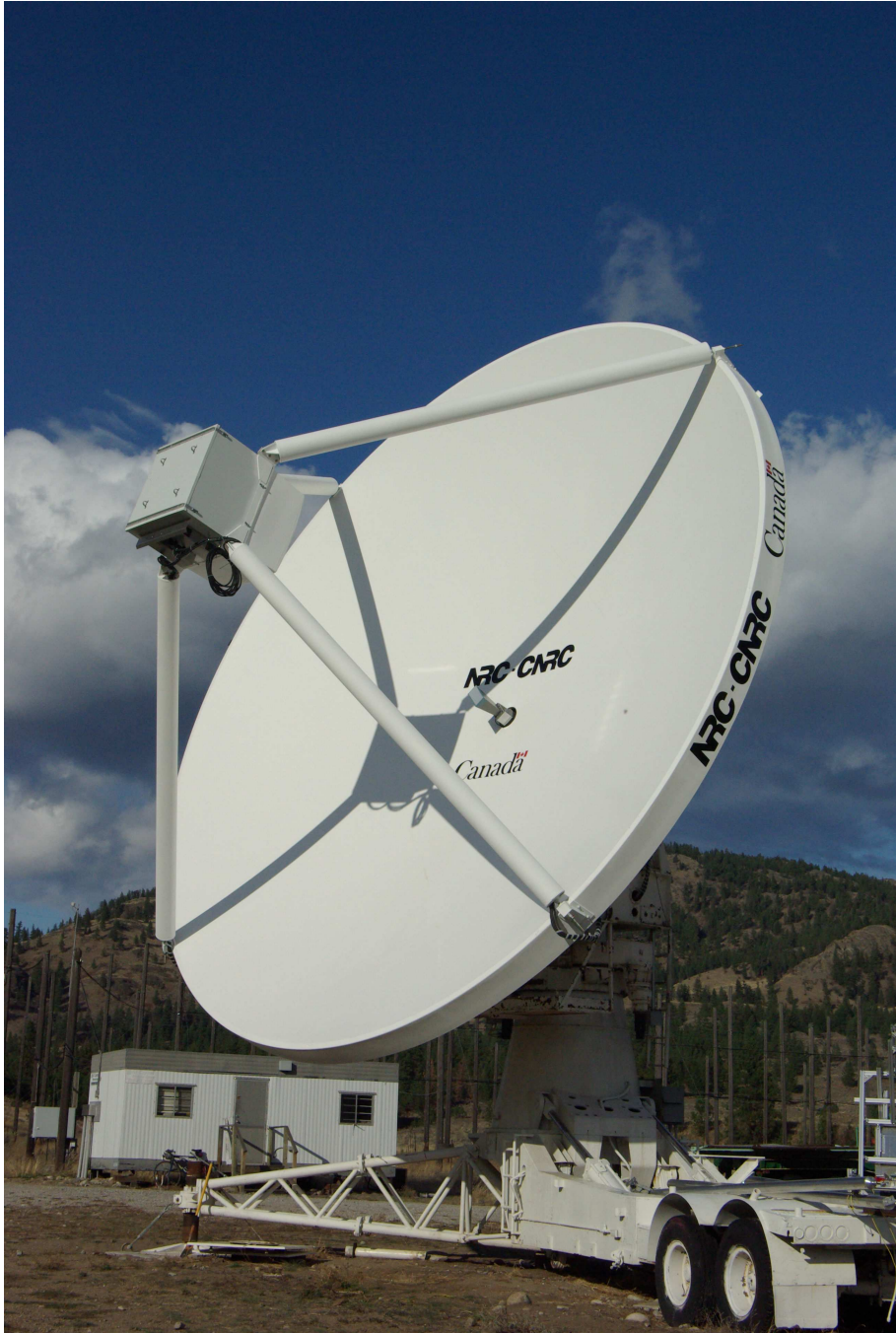
Figure 1. Second prototype 10 m composite antenna at DRAO being used to test focal plane array.
