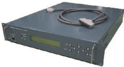
Figure 1. The ADS2000 can sample 16 baseband channels at the sampling rate of 64 Msps suitable for the bandwidth synthesis.
