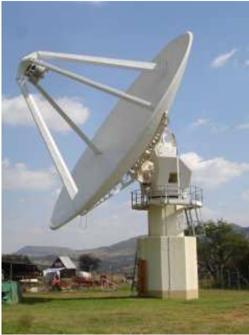
Figure 2. 15-m XDM: the KAT prototype is to be converted to a radio telescope capable of performing geodetic VLBI experiments. (Credit: M. Gaylard)
