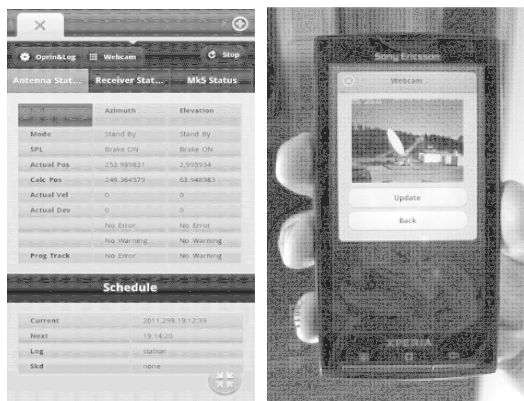
Figure 4. (left) A screen shot of the smartphone software with Antenna Control Unit and the current schedule. (right) Webcam of the radio telescope in the interface of the smartphone software for VLBI experiments.
