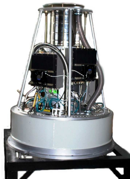
Fig. 1 Tri-band receiver focal container (without housing).
