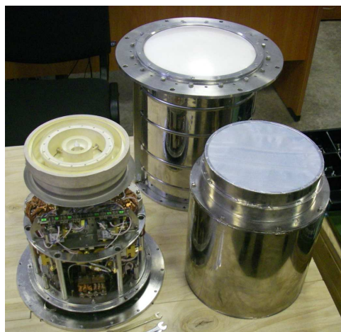
Fig. 2 Cryostat assembly: equipment, container with vacuum window, thermal screen.
