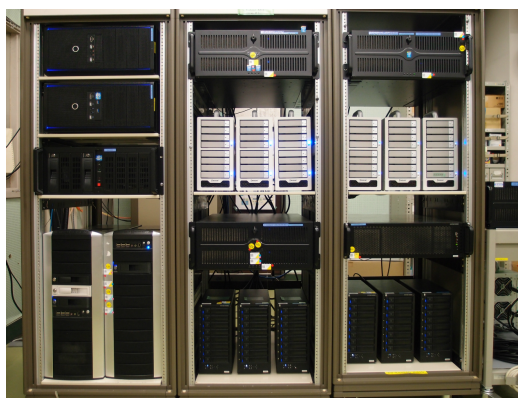
Fig. 1 Correlators of NICT/Kashima using the GICO3 software correlator.
