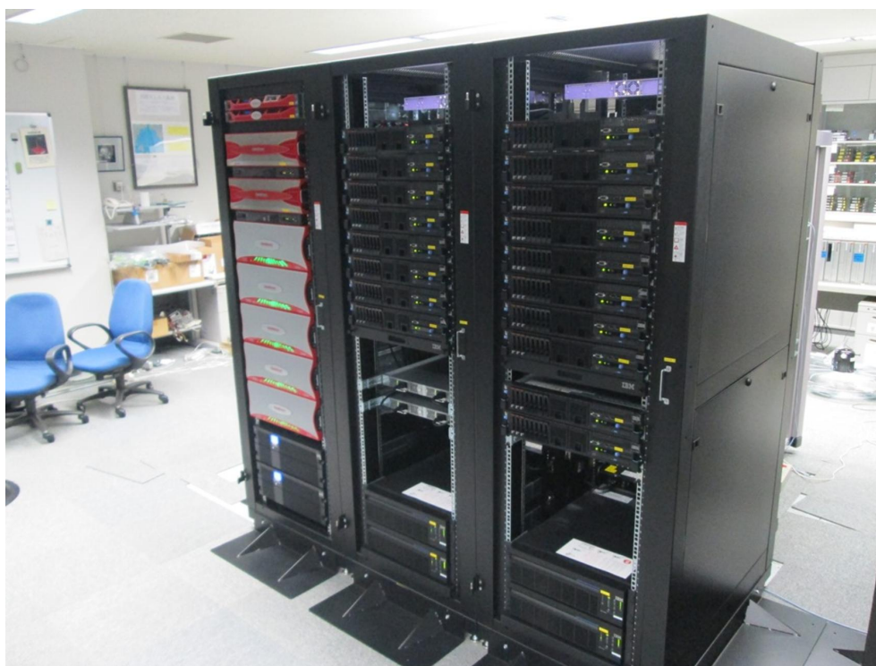
Fig. 1 View of the main system (data processing servers and storage) at the Tsukuba VLBI Correlator.
