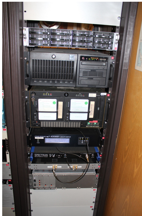
Fig. 3 The new data acquisition rack with (from top) backup system, Field System PC, Mark 5B+ data recorder, and ADS3000+ gigabit sampler.
