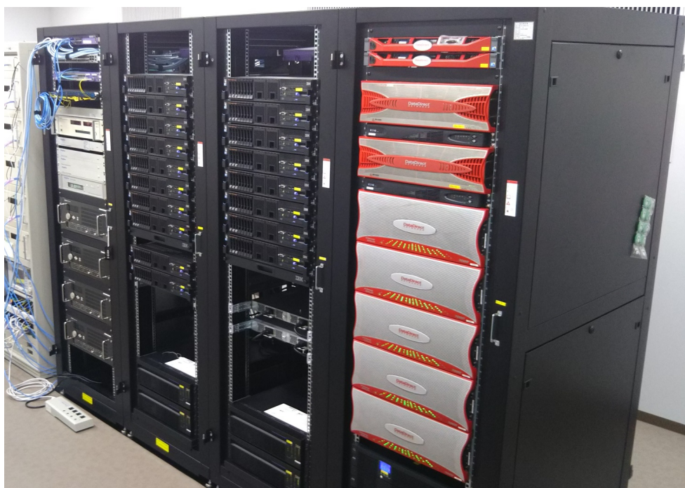
Fig. 1 View of the main system (data processing servers and storage) at the Tsukuba VLBI Correlator.
