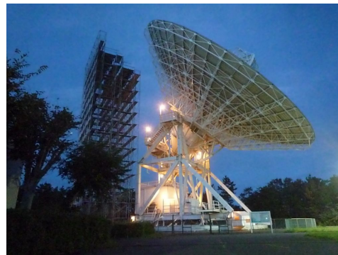
Fig. 6 The Kashima 34-m antenna in holographic observing after reflector adjustment. We carried out the reflector adjustment during day time and the holography observing in the evening. We repeated this procedure for a week. For safety, we watched the antenna during the holography observing for about 1.5 hours to avoid an accidental smash with the scaffolding.
