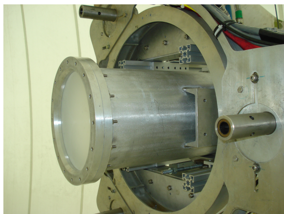
Fig. 2 View of the Westford antenna VGOS feed which is located at prime focus on the antenna.
