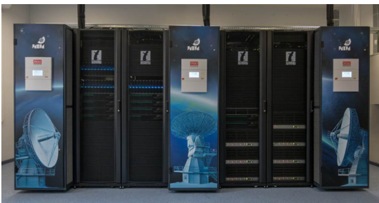
Fig. 2 RASFX GPU-based software correlator.
