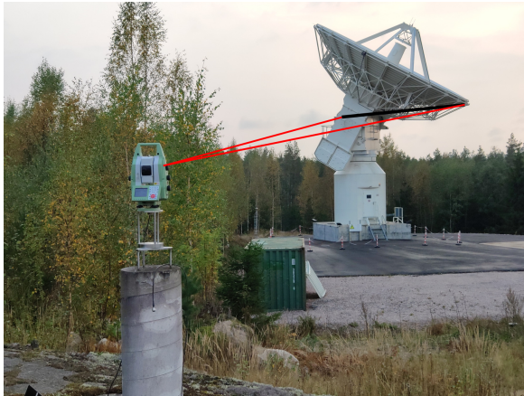
Fig. 1 Measurements with Leica TS50 robot tachymeter.
