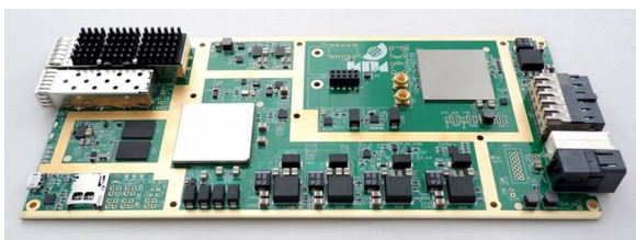
Fig. 2 The DSP unit shown with the heat sink removed.
