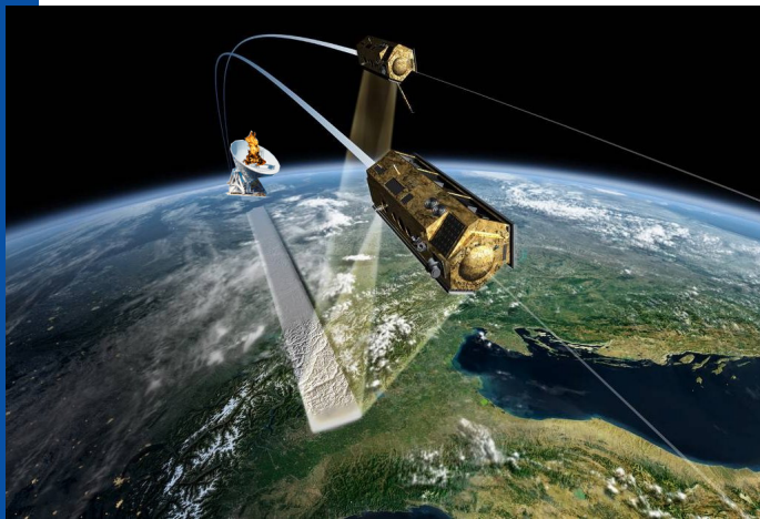
Exaggerated depiction of a saturated (or 'fried') frontend of a radio telescope due to an SAR transmission.
