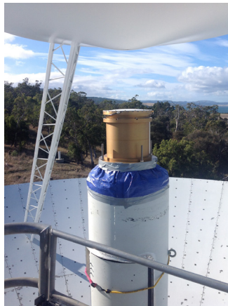
The Callisto VGOS receiver mounted with preliminary weather protection on the Hobart 12-m antenna.
