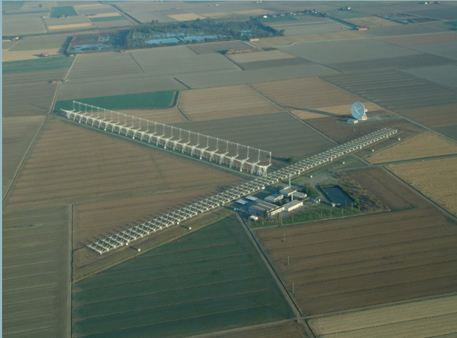
Aerial photo of the Radio Astronomical Observatory of Medicina (Bologna) with the Northern Cross in the foreground and the 32-m diameter VLBI antenna in the background. The Northern Cross is a transit instrument working at a wavelength of 73.5 cm (or 408 MHz).
