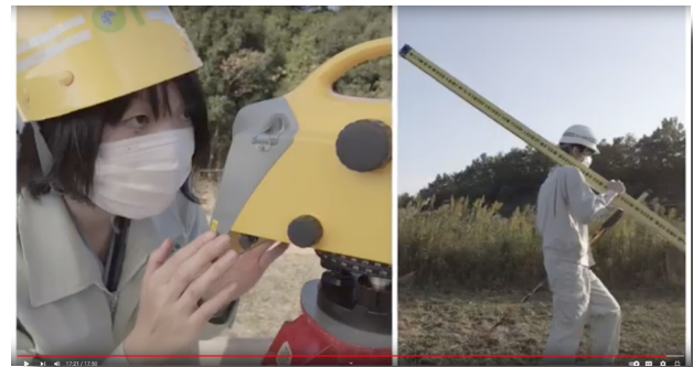
(From GSI's video about local-tie survey) Determining local height differences with geometric leveling.
