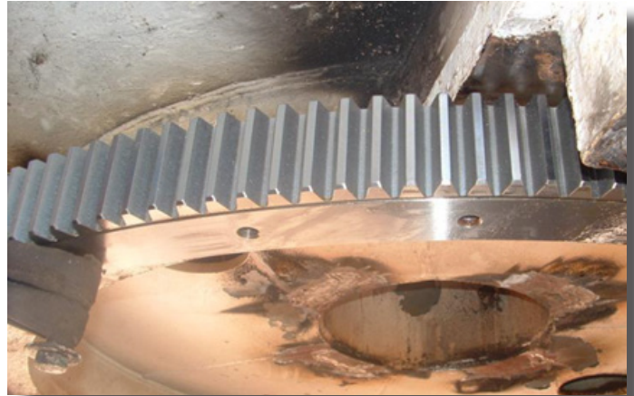
New Azimuth Bearing following Installation.
