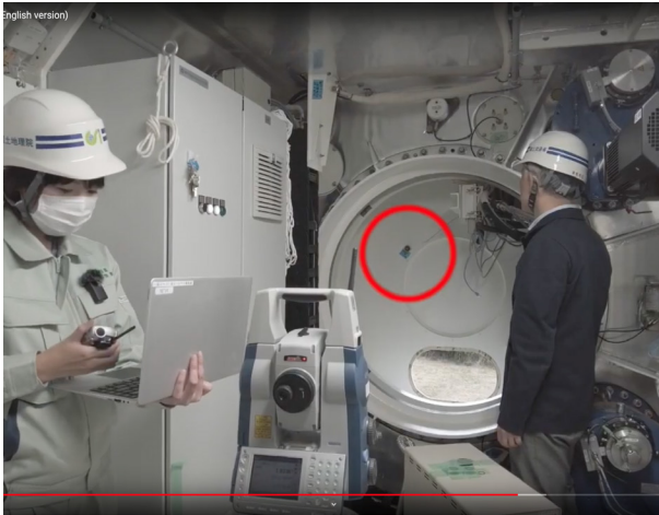
(From GSI's video about local-tie survey) Determining the VLBI reference point of the Ishioka antenna by measuring distances and angles to a target on the moving dish using a total station that is physically fixed to the ground.
