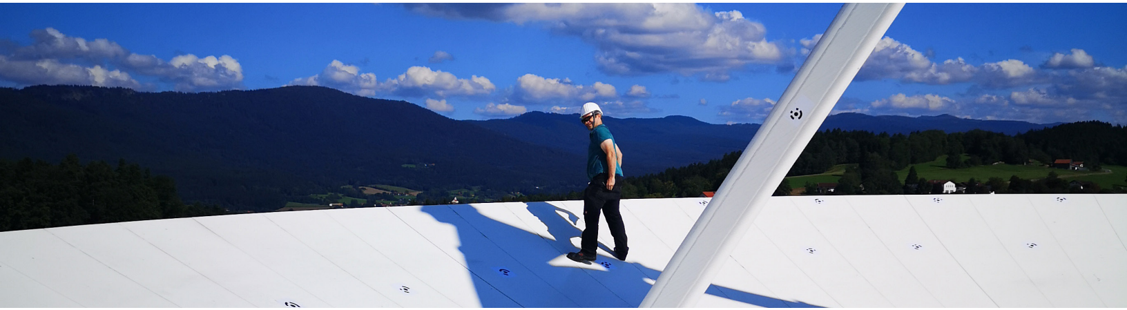
Alexander inspecting the photogrammetric markers in the antenna.
