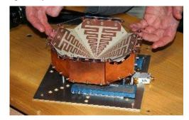
**Fig. 4.** Prototype of a broadband 2-14 GHz "Eleven" feed for VLBI2010. The feed is being developed at Chalmers University in Sweden.
