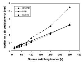
**Fig. 1.** Median of the rms 3D position errors for uniform sky schedules with regular source-switching intervals ranging from 15 to 360 s. The delay measurement noise is 4 ps per baseline observation, the clock Allan Standard Deviation is  $1 \cdot 10^{-14}$ @ 50 minutes, and the turbulence parameters are those driven by a turbulence model (Petrachenko et al., 2008).
