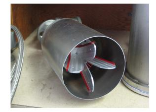
Fig. 2. The ETS-Lindgren quad-ridge broad band feed-horn (ETS-Lindgren, 2007) inside a heat shield attached to the 15 K station of the cryogenic refrigerator. The dewar is on the right hand.
