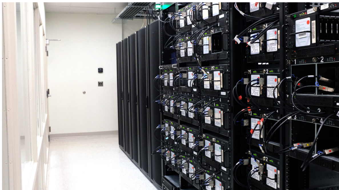
Fig. 1 (Background) Cluster correlator and (foreground) Mark 6 playback units at the MIT Haystack Observatory.
