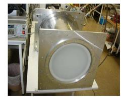
Figure 3. Preliminary results: measured system noise temperature of Eleven feed in cryostat at 28 K physical temperature (left picture) and Eleven feed prototype mounted in the test cryostat with 4-8 GHz cryogenic LNAs.
