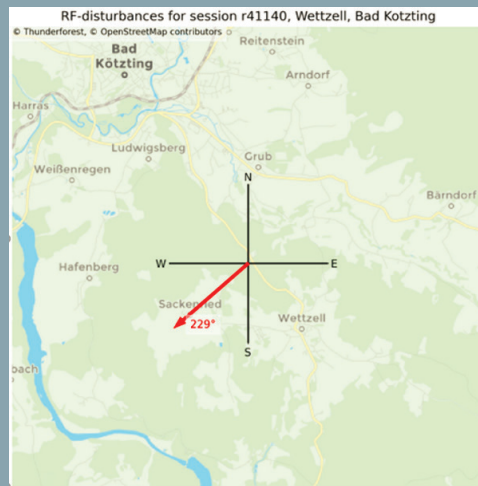
Sample map with strongest RFI source during an R4, pointing to a local mobile communication sender
