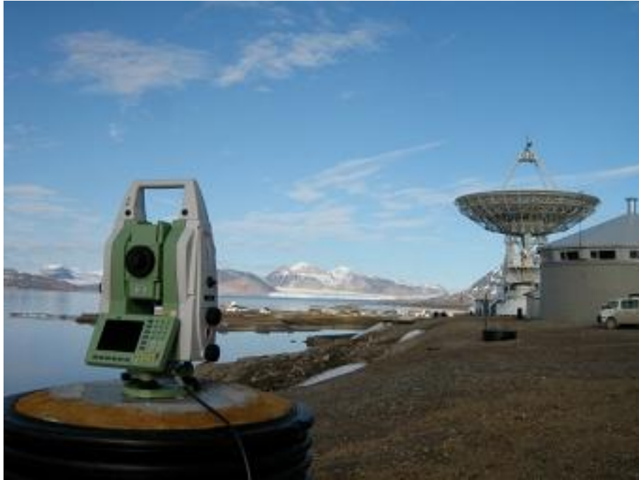
The TM 30 on survey pillar P93.
