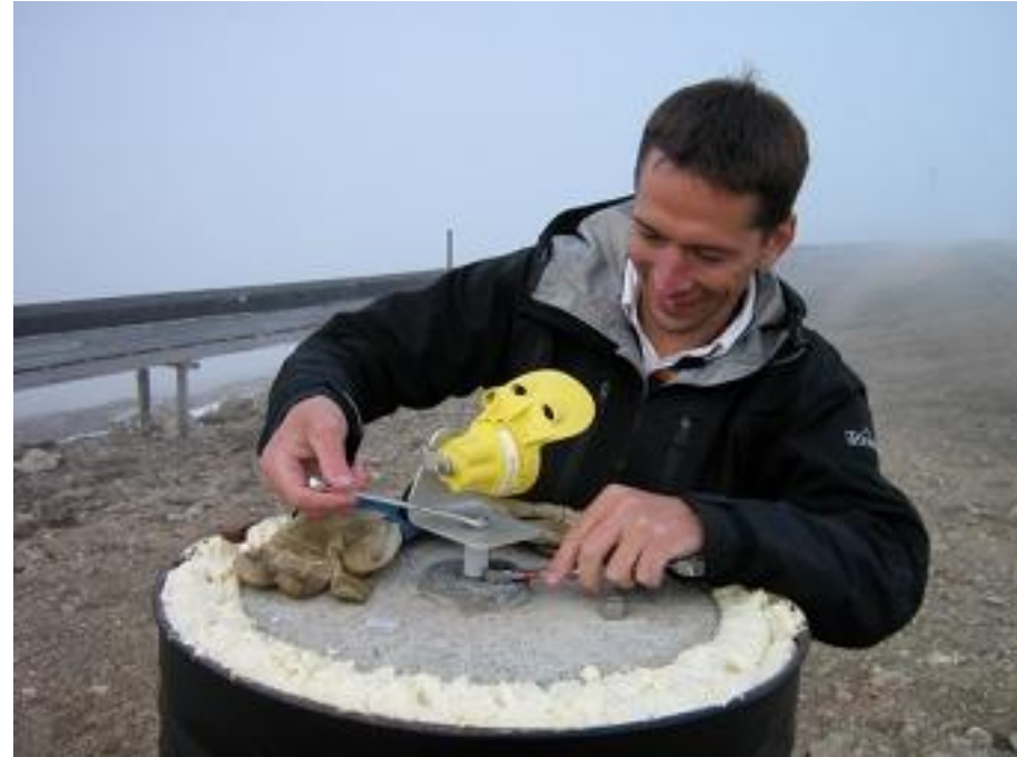
A prism on one of the survey pillars.
