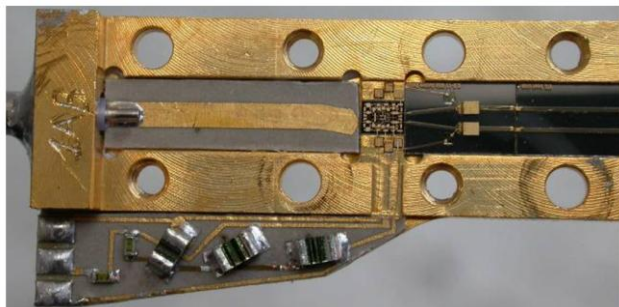
The active cryogenic balun developed at Caltech mounted in module.
