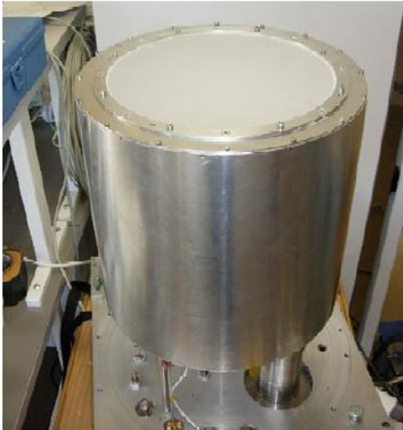
The 70K shield has infrared window of one layer Teflon
