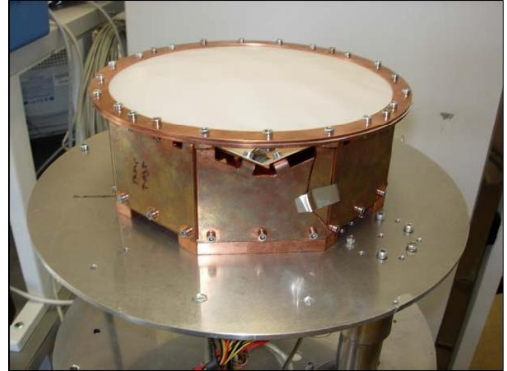
The infrared filter in front of the Feed has only two layers of Teflon separated by wedding veil. The temperature on the surface of the petal was 53K.
