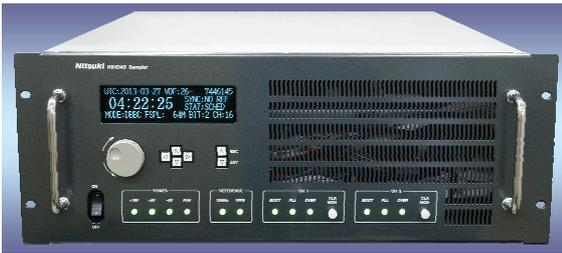
Fig. 9 K6/iDAS VLBI Sampler.
