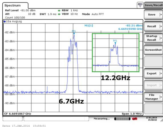
**Fig. 3** Methanol maser emission at 6.7 GHz and 12.2 GHz from W3OH were observed simultaneously with broadband feed (IGUANA-H) of the 34m antenna.
