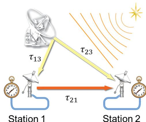
Fig. 1 Concept of GALA-V project for distant frequency comparison.
