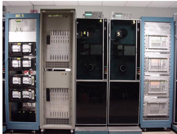
Figure 1. Partial view of the Haystack Mark IV correlator, showing 1 rack containing 4 Mark 5A units and a decoder, correlator rack, 2 tape units and 1 rack containing 4 station units.
