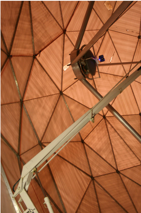
Fig. 3 Laser scanning of antenna dish. The scanner is in place of the secondary mirror.
