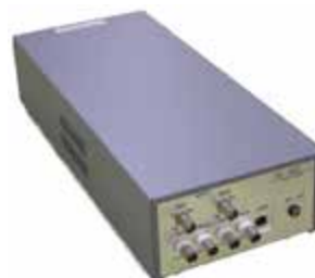
Fig. 3 One unit of K5/VSSP32 sampler has four video signal inputs. Data output and remote control is made via USB2.0 interface. One geodetic terminal of 16 video signals is composed of four units of this device.
