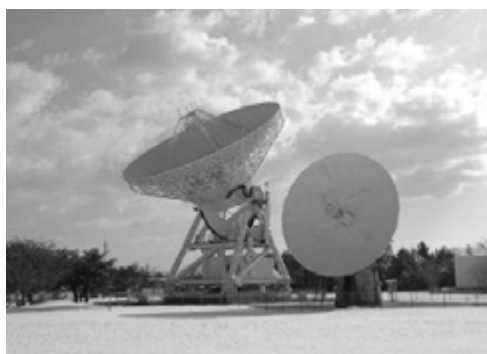
Fig. 1 The front view is of the Mizusawa 10-m antenna, and the back view is of the VERA Mizusawa 20-m antenna.
