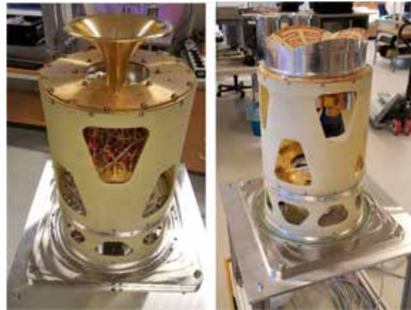
Fig. 3 The interior of the two OTT cryogenic receivers with QRFH (left) and Eleven-Feed (right).
