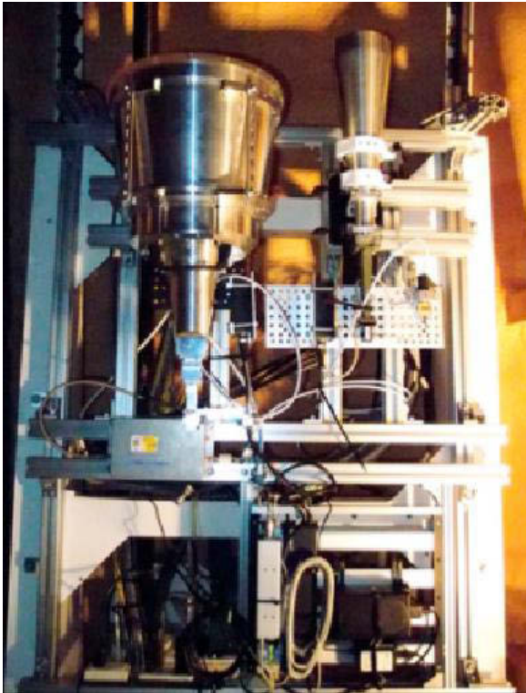
Fig. 1 NINJA feed (left) and IGUANA feed (right) in the feed cone of the Kashima 34-m antenna.
