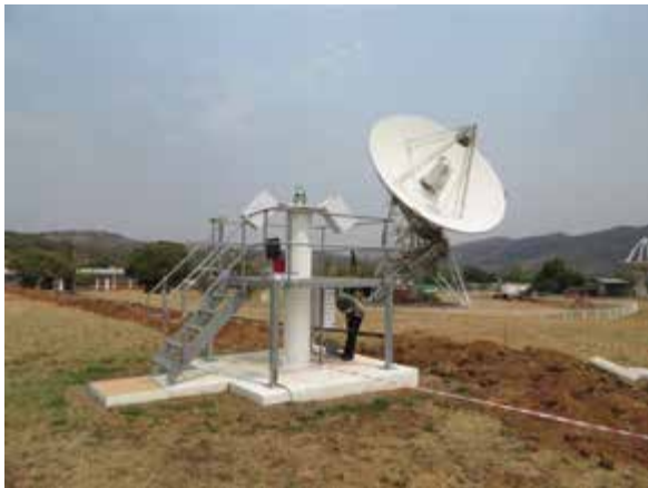
Fig. 5 The local automated site tie system is nearly ready to start operations.
