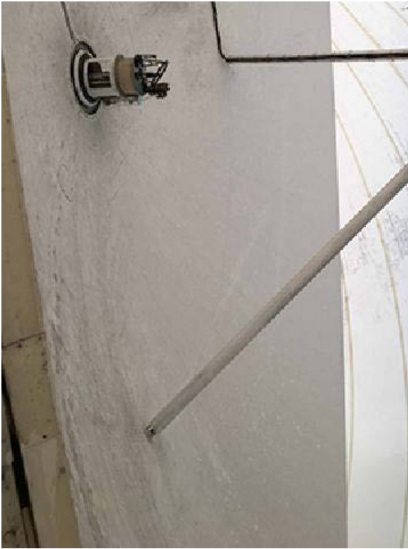
Fig. 2 View of the Westford antenna inside the radome. The VLBI VGOS receiver is located at the prime focus.
