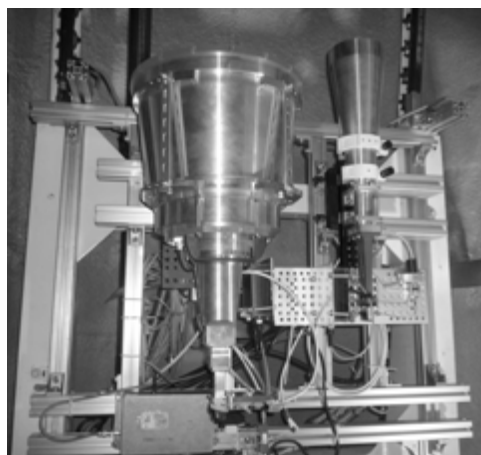
Fig. 2 A broadband NINJA feed was installed in the receiver room of the Kashima 34-m telescope.
