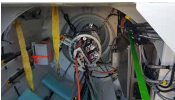
Fig. 2 Signal Chain frontend deployed at KPGO (focus cone).
