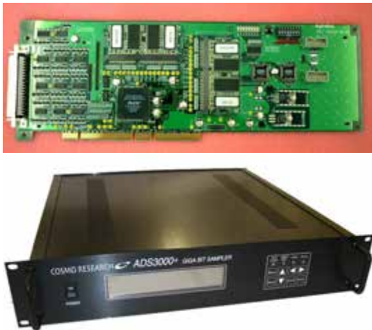
Fig. 4 Upper panel shows PC-VSI card, which captures VSI-H data stream. Up to 2048 Mbps data stream is captured by one interface card. Lower panel shows ADS3000+, which is capable to extract 16 channels of narrow band signals via DBBC function, and it outputs data stream through VSI-H interface.
