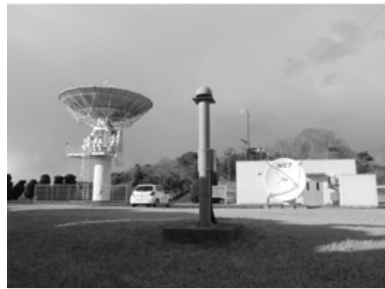
Fig. 5 The Kashima 11-m antenna and the GNSS receiver pillar of the IGS tracking station KSMV.
