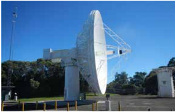
Fig. 1 Newly installed 12-m VGOS telescope at KPGO.
