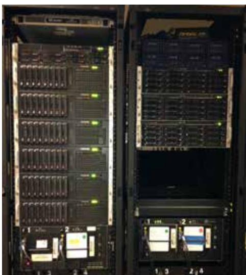
Fig. 1 Partial view of the Haystack DiFX correlator, showing two racks containing seven computer servers, three file storage servers, one Qlogic infiniband switch, and two Mark 6 playback units.
