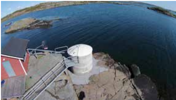
Fig. 2 The Onsala super tide gauge inaugurated in September 2015 and since then operated together with SMHI.
