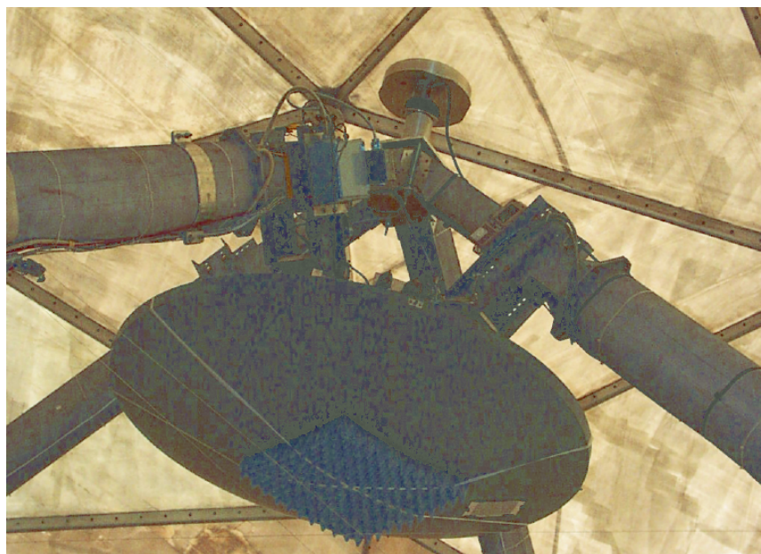
Figure 1. APEX antenna on top of the subreflector support structure.
