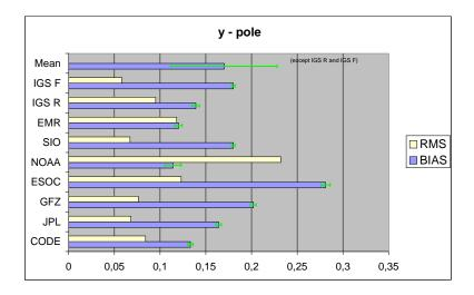
Figure 2. Biases and rms of GPS operational series with respect to C04: x-pole, y-pole.
