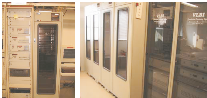
Figure 1. K-4 VLBI observation system at observing stations (left) and K-4 correlator system at Kashima Space Research Center (right).
