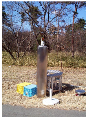
Figure 1. GSI Ground Monument
