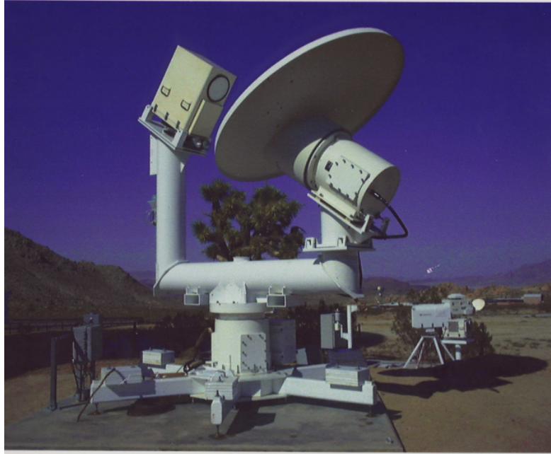
Figure 1. A photo of the Cassini calibration subsystem taken at DSS-13 in Goldstone CA. The new advanced WVR is seen in the center and the MTP and J-series WVR are shown in the background to the right.
