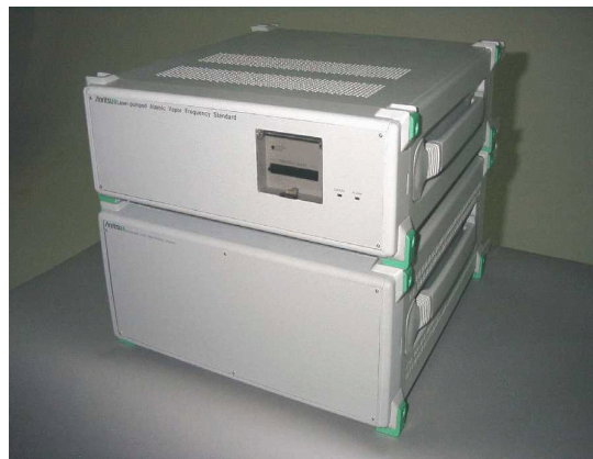
Figure 2. Photograph of the developed atomic clock. The 1-MW 7"-high module on the bottom contains the physics unit coupled with the light frequency-stabilized LD and most of the electronic circuits. The 1-MW 5"-high module on the top contains the frequency-adjustment digital switch, a CPU, and power supplies.
